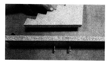
1) In the 18" wide 14 sample board box find the 2 - 18" back rail with 2 holes, 2 - step blocks and 2 confirmat screws(in hardware bag). Make 1 left hand and 1 right hand (Left hand shown). Screw the 2 pcs together.
